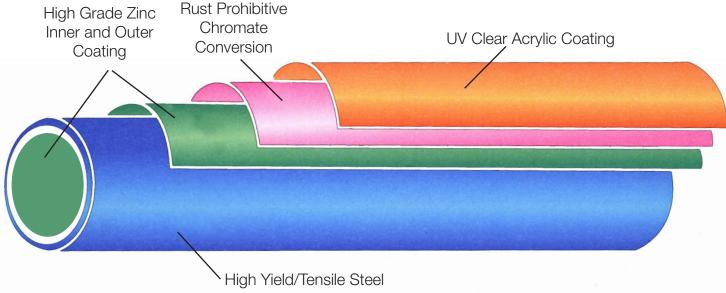
Iron World's industry leading galvanized clear coat process for fence framework:
